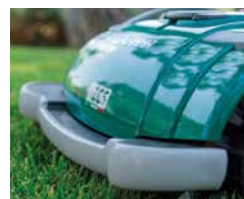
Parachoques y sensor de obstáculos Bumper and obstacle sensor
